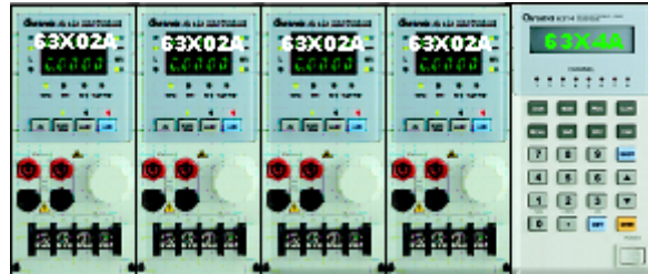
Figure 4-4 Indication of Channels
